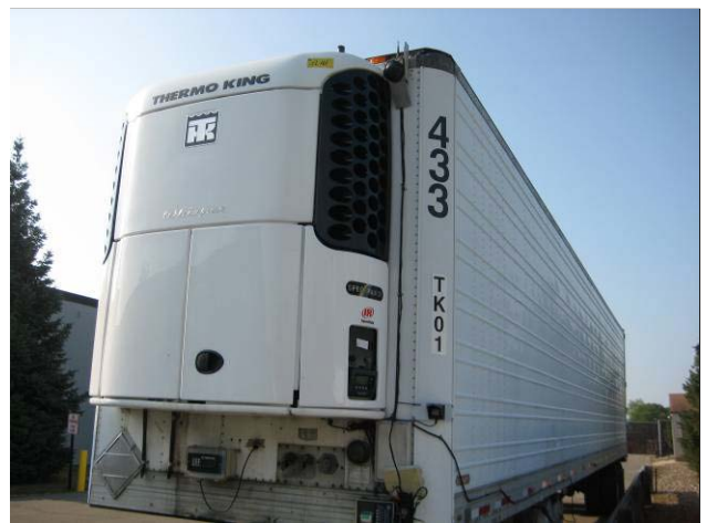
Figure 1. TRU Mounted on Trailer Nose
